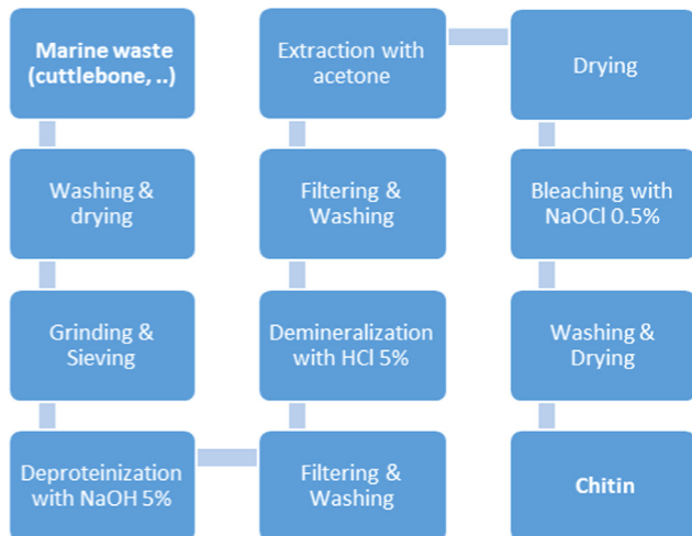
Fig. 2. Overall process for preparation of chitin from cuttlebone.
